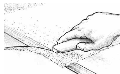
Figure 26 Trim excess cloth after the epoxy gels.
